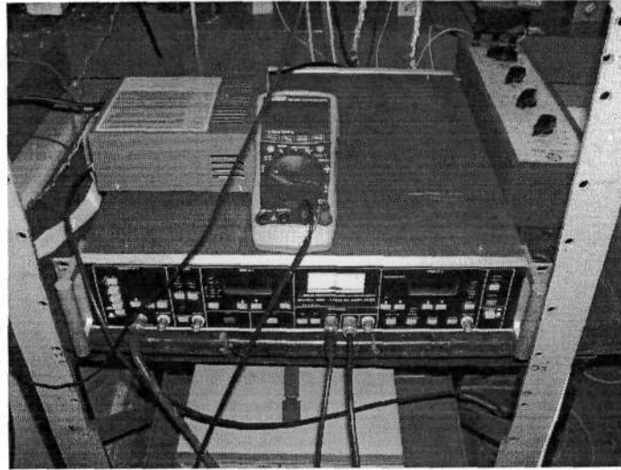
Figure 5.14: Photo of the phase-sensitive Detector
