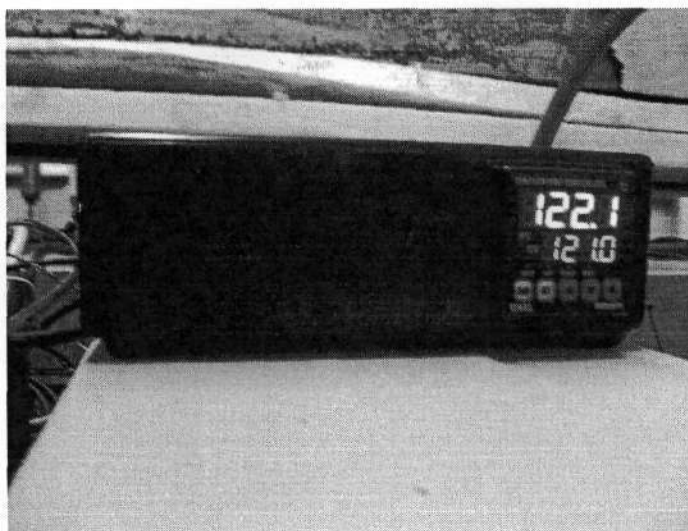
Figure 5.19: Photo of the new temperature controller
