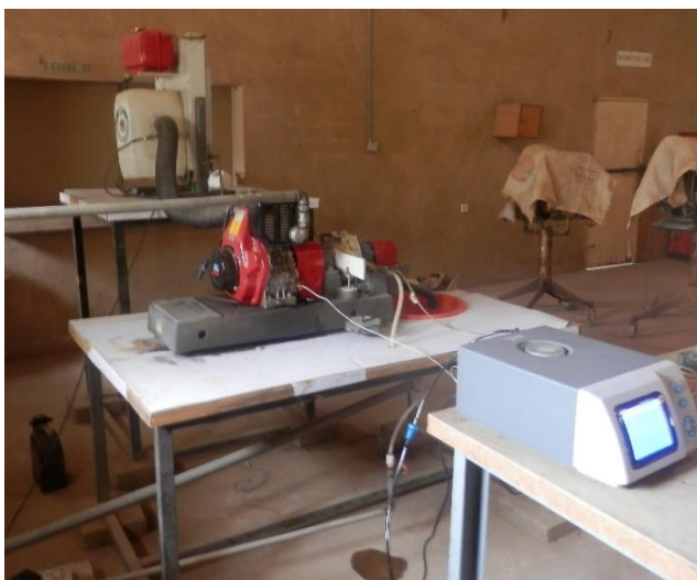
Plate 1: CI Test rig showing emission measuring device
