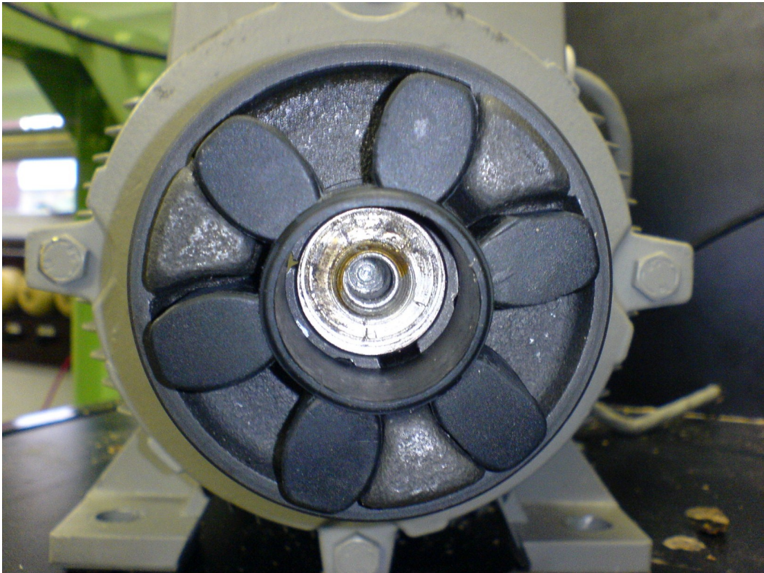
Figure 5-16 Photograph showing metal coupling with a rubber insert, with new rubber insert that provides for minimal gear play
