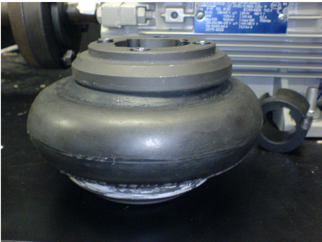
Figure 5-14 Photograph of tire type coupling used to emulate a coupling with elasticity or flexibility
