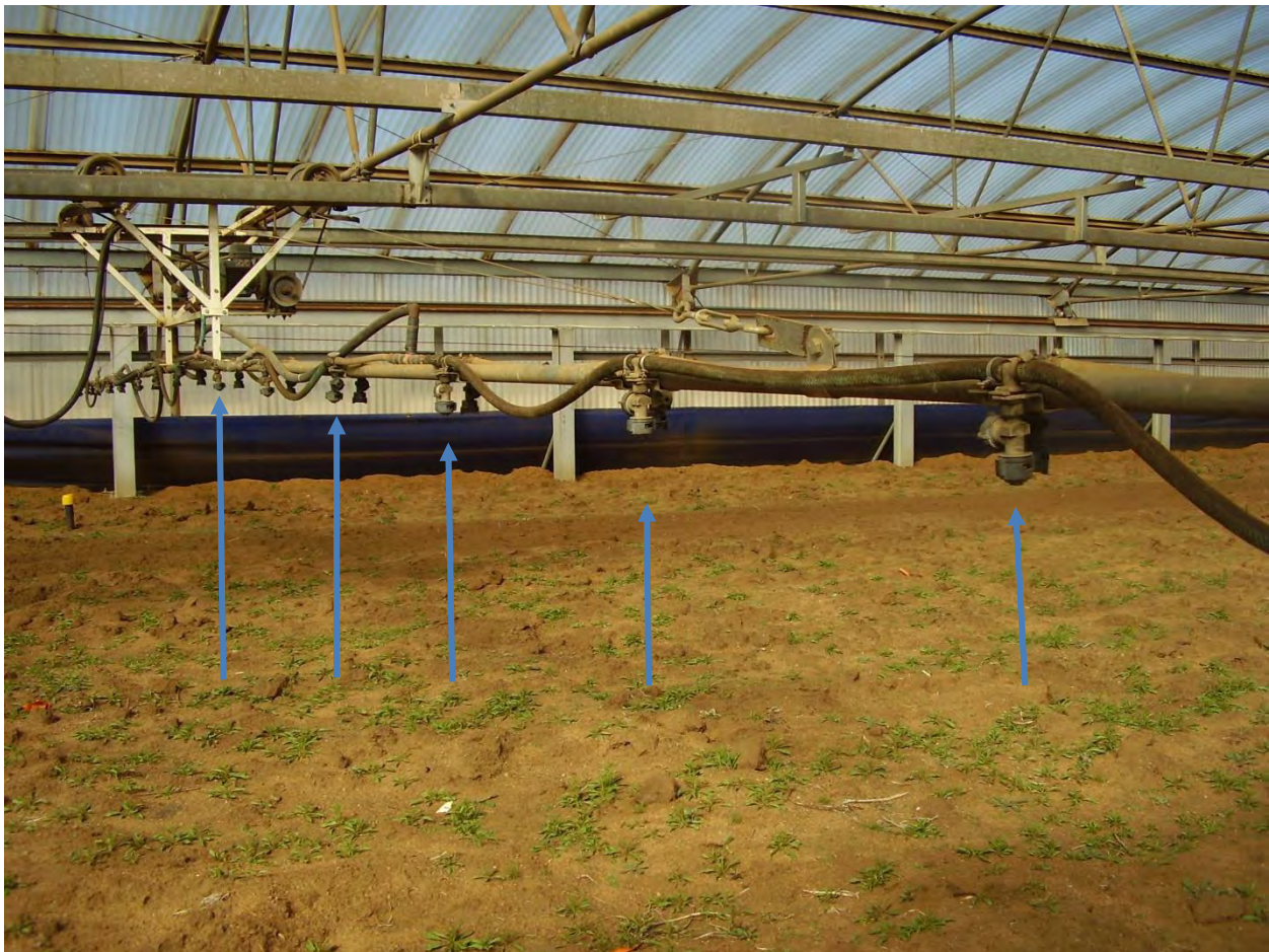
Figure 2.4: Irrigation boom in large rainout shelter for the supply of various irrigation quantities. Blue arrows indicate some nozzle locations.
