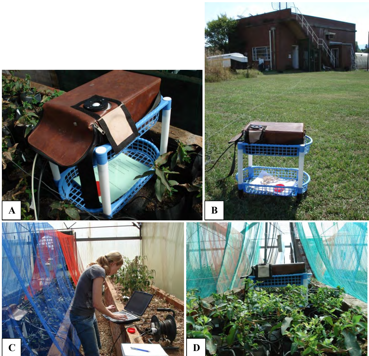
Figure B.6. Using the spectroradiometer (A) in the stock plant tunnel showing the sensor on top, (B) outside away from buildings and plants. (C) Setting the parameters on the computer and (D) the spectroradiometer was placed above the stock plants to avoid reflection off leaves that can lead to false readings.
