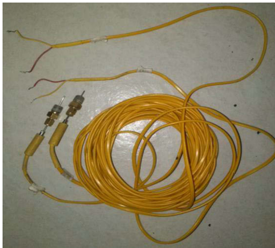
(a) Type-K thermocouple pipe
