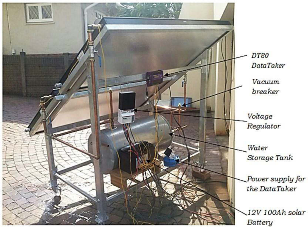
Figure 47: The rear view of the experimental set up
