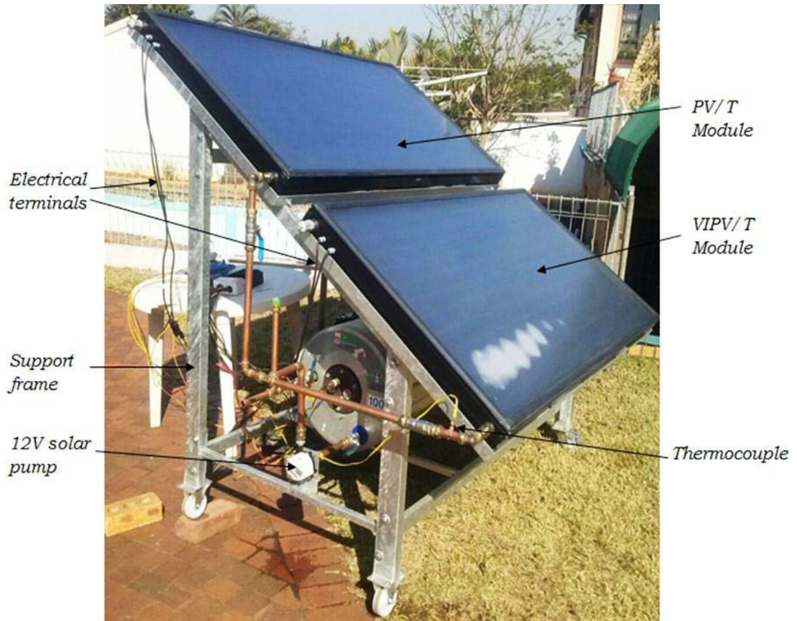
Figure 46: The front view of the experimental set up
