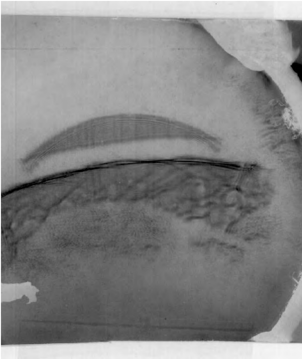
Figure 4.1.5.: The single strong shock coming from the coil, probably due to the jumping of the arc across the coils.
