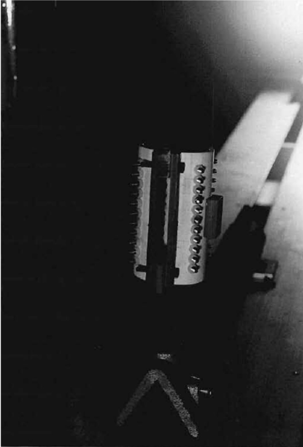
Figure 4.1.1.: Cylindrical shock generator by a series of spark gaps in series from Kuppen [2]
