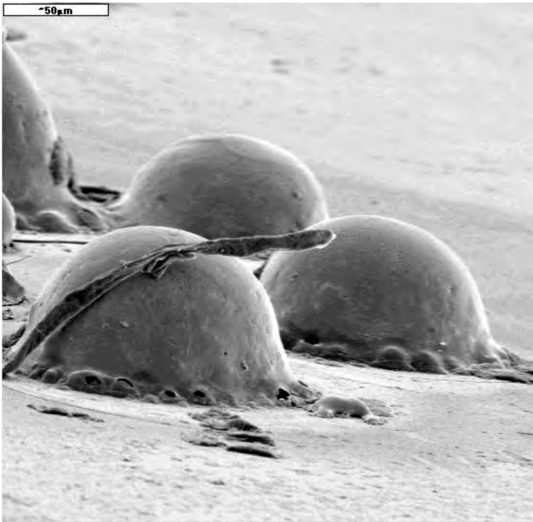
Figure 4.5.1.: SEM pictures of droplets of melted wire on the lens.
