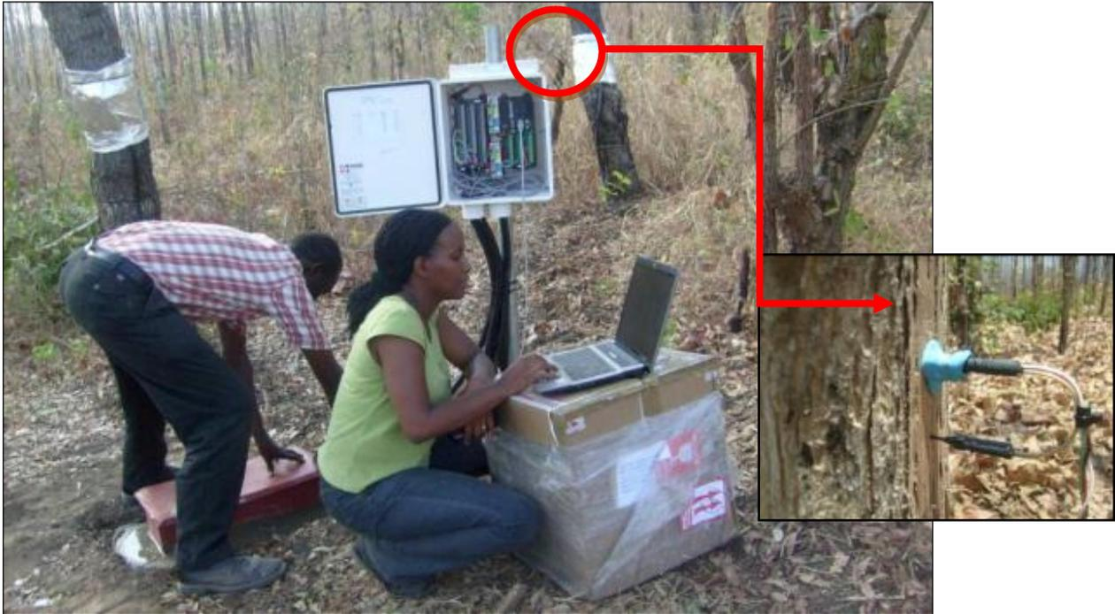
Figure 3.7 Installation of TDP sensors within the Miombo forest, adjacent to the Teak forest plantation (lower photo shows: silicone covering the exposed part of the TDP probes: upper heated needle and lower reference needle)
