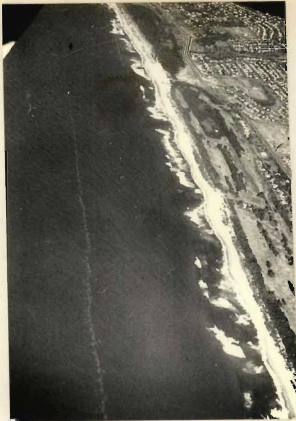
Photo 3.1. Line of dye laid parallel to the coast - Virginia Beach.
