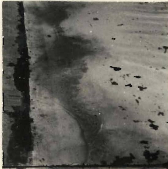
Photograph 3.20. Oblique photograph (looking along the water's edge) of two edge waves travelling in opposing directions and forming a standing wave - which is marked with dark dye.
