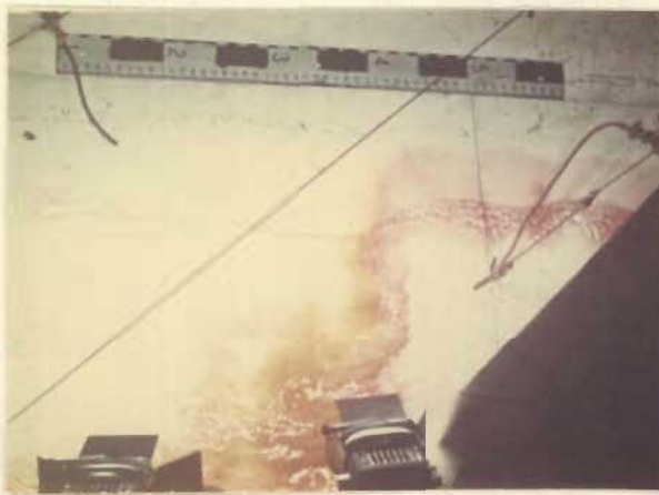
Photograph 3.6 detail of a large rip current in the model with small rips in the red dye.
