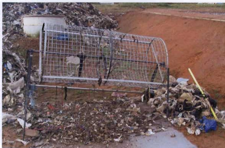
Plate 1 Waste sample sieving process at the Bisasar road landfill site.
