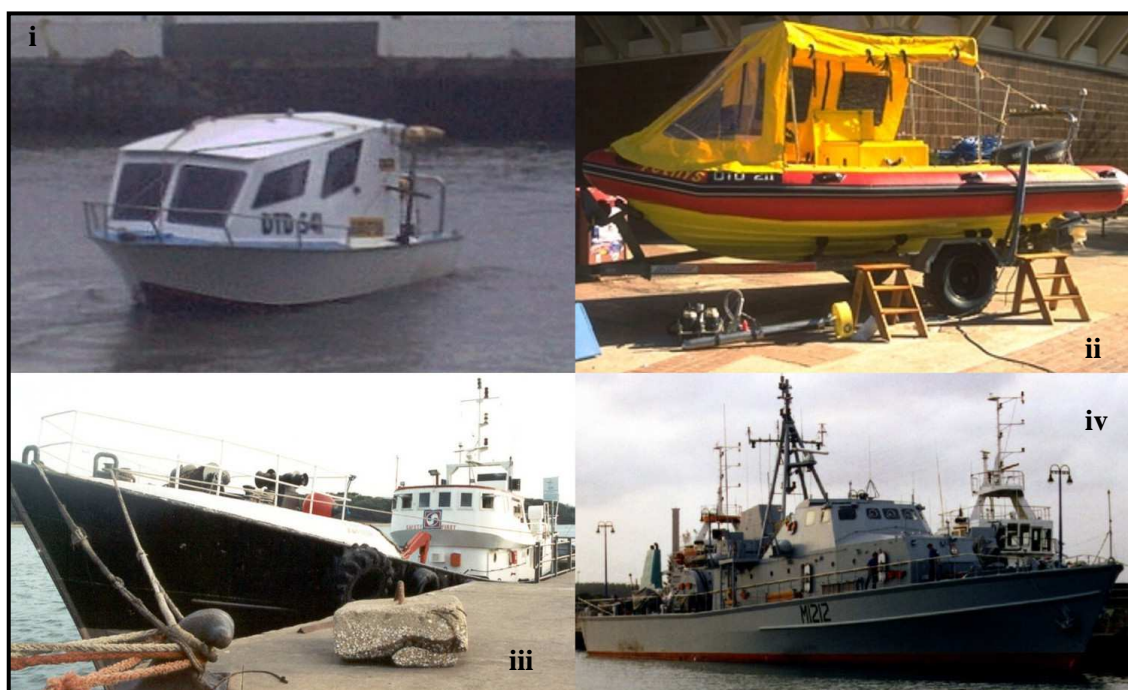
Figure 5.2 Vessels used to collect the geophysical data for this study. i) Subtech Surveyor , ii) Tethys , iii) MV Ocean Mariner and iv) SAS Umhloti . The skiboats Tethys and the Subtech Surveyor were used because of low cost, suitability for beach launching and rapid deployment.
